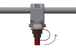
2. Watermist will release into the engine compartment.
