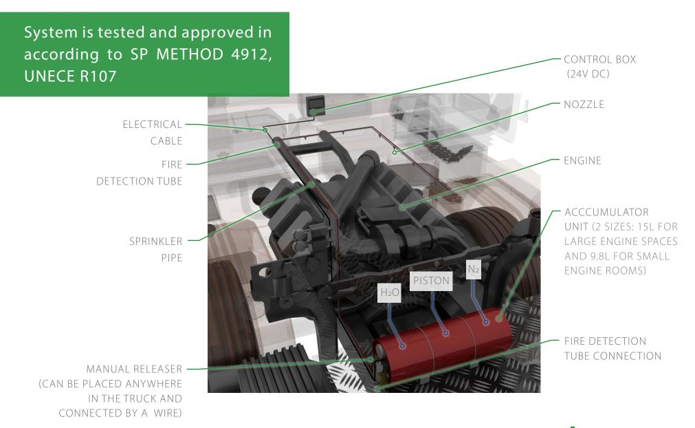
Vehicles System Protection Scheme The accumulator unit consists of two chambers - the first contains compressed gas, and the second is filled with fire extinguishing liquid water. A piston separates the two sections.
