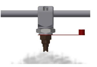
3. After activation and extinguishing process, nozzle cover has to be put back in place, covering the nozzle.
